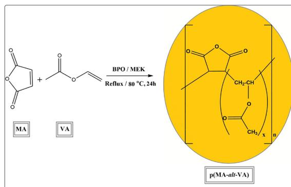
Scheme 1. Synthesis reaction representation of pMAVA copolymer.
