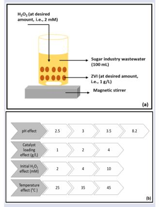
Figure 1. Experimental set-up (a) and reaction conditions (b)
