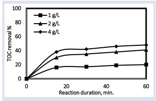
Figure 3. ZVI loading effect (Reaction conditions: 100 mL sugar industry wastewater, pH: 3.5, ZVI: 1-4 g/L, [H<sub>2</sub>O<sub>2</sub>]<sub>0</sub>: 2 mM, T: 25 °C t: 60 min)
