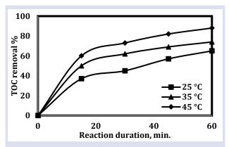
Figure 5. Temperature effect (Reaction conditions: 100 mL sugar industry wastewater, pH: 3.5, ZVI: 2 g/L, [H<sub>2</sub>O<sub>2</sub>]<sub>0</sub>: 4 mM, T: 25-45 °C t: 60 min)
