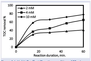
Figure 4. Initial H<sub>2</sub>O<sub>2</sub> effect (Reaction conditions: 100 mL sugar industry wastewater, pH: 3.5, ZVI: 2 g/L, [H<sub>2</sub>O<sub>2</sub>]<sub>0</sub>: 2-10 mM, T: 25 °C t: 60 min)
