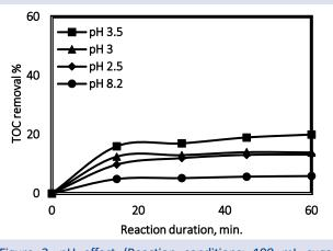
Figure 2. pH effect (Reaction conditions: 100 mL sugar industry wastewater, pH: 2.5-8.2, ZVI: 1 g/L, [H2O2]0: 2 mM, T: 25 °C t: 60 min)
