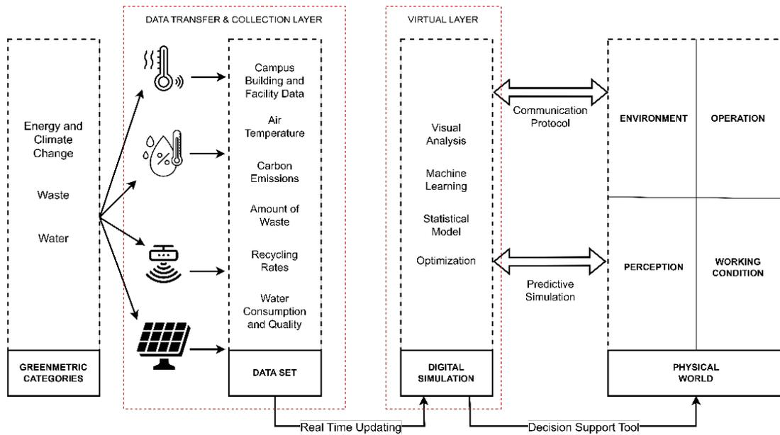
Figure 3. Conceptual Framework Design of Digital Twin for GM Criteria in Smart Campuses
