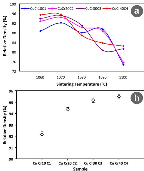
**Figure 2.a)** Change of relative density with sintering temperature in the produced composites, **b)** Obtained relative density values by sintering at 1070 °C
