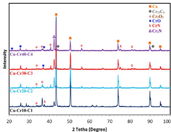
**Figure 3.** XRD diffraction patterns of the produced composites
