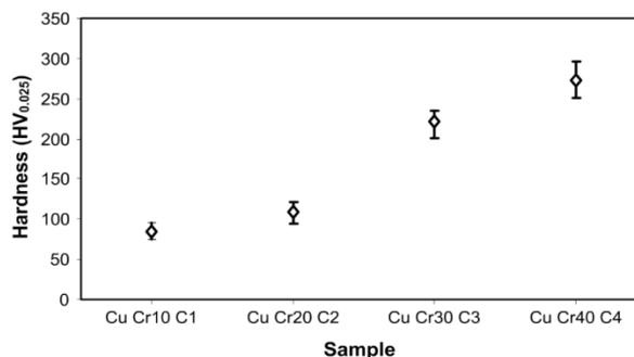
**Figure 6.** Hardness values of the produced composite samples
