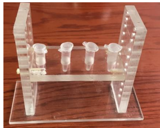
Figure 1. Phantom and simulated lesions (tubes).
