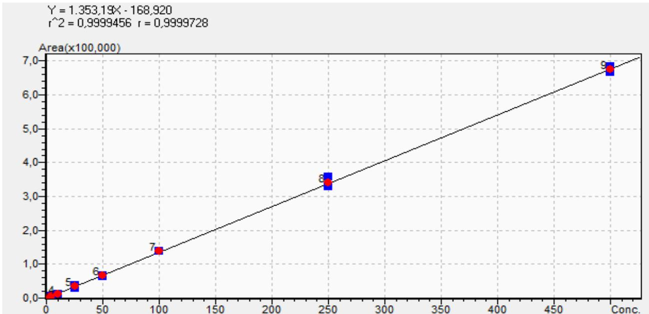
**Figure 3.** Nine point of calibration curve with linear correlation.
