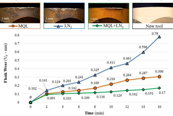
Figure 6. Flank wear results (at 180 m/min cutting speed, and 0.1 mm/rev feed rate) (Maksimum yanak aşınma sonuçları (180 m/dak kesme hızı ve 0.1 mm/dev ilerlemede))
