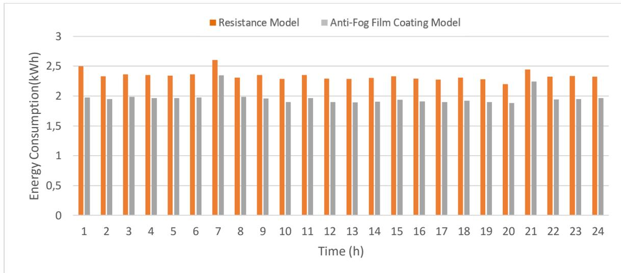
**Figure 5.** Energy consumption of the refrigeration system
