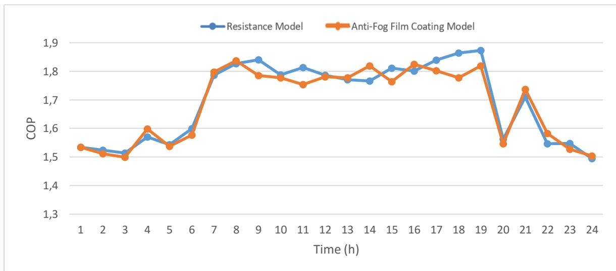
**Figure 6.** COP value of the refrigeration system
