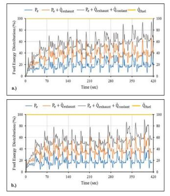
Figure 6 Instantaneous energy distributions of fuel energy at 2000-3000 rpm / 25% load, [a.) MPICS - b.) EPICS].
