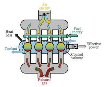
Figure 2 Input and output energy terms for control volume of the engine.
