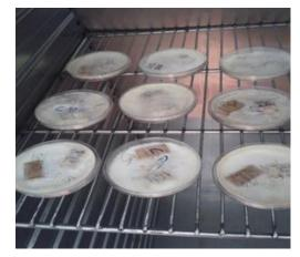
Figure 1. Fungal decay test
