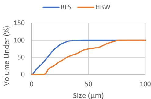
**Figure 1.** Sieve analysis of the BFS and HBW
