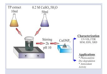
Figure 1. Schematic diagram of the green synthesis of CuO NPs
