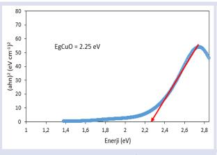
Figure 4. Optical energy band gap of CuO NPs
