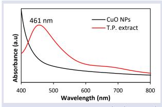
Figure 3. UV-Vis UV-vis spectroscopy absorbance results of TP extract and CuO NPs
