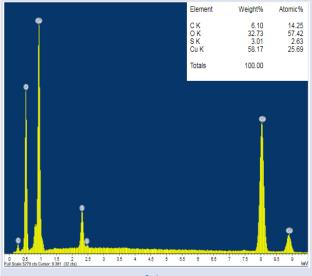
Figure 7. EDX spectrum of the CuO NPs
