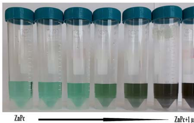
Figure 2: The color change of ZnPc-GO hybrids at different concentrations (GO concentration increases from left to right).
